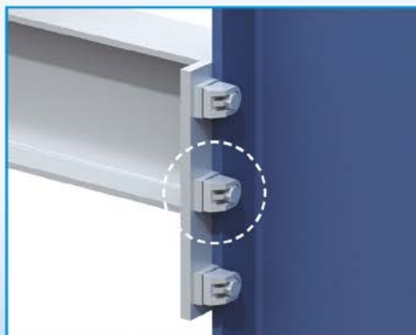
Beam-to-column (slip resistance)
