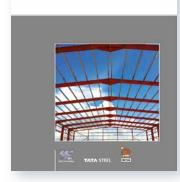
Steel portal frames account for around 50% of the structural steel used in the UK and are firmly established as a light weight, cost effective and efficient way of enclosing usable volumes in construction.
