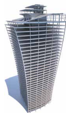
To balance the structure the main core was moved slightly off centre during the design model stage
