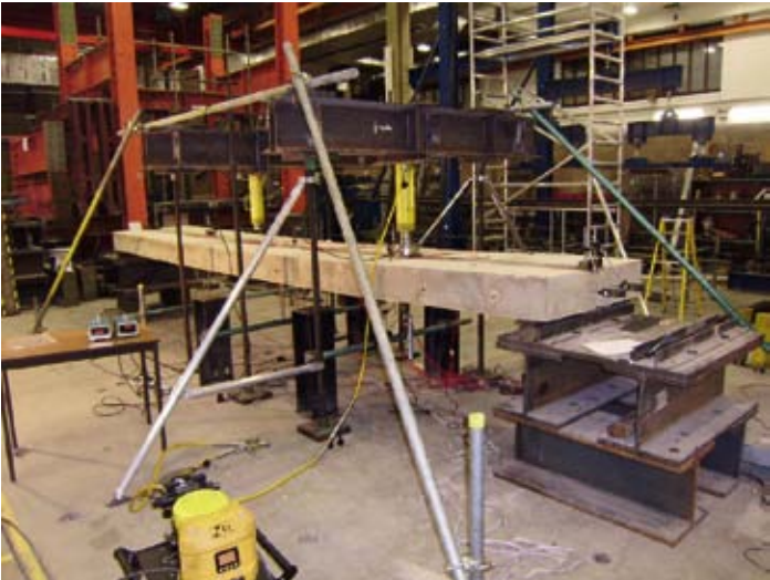
Figure 2: USFB® Test 2 at City University showing the single off centre load point
