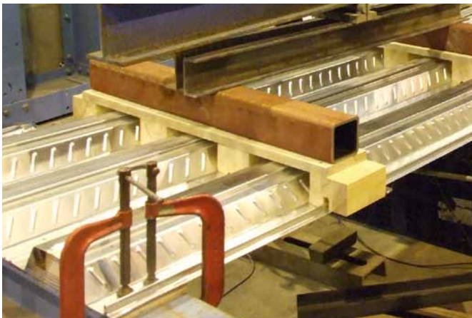
Single-span sagging test at the University of Salford.
