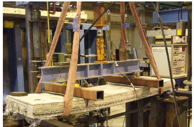
Composite slab test at the University of Salford.
