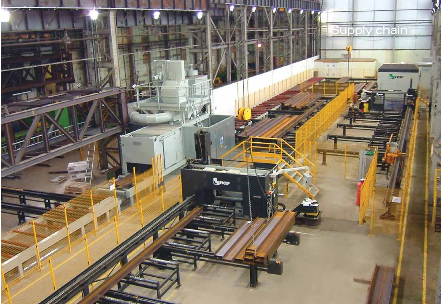
Above: Ficep Automatic CNC machines with scribing facility at Elland Steel's yard.
