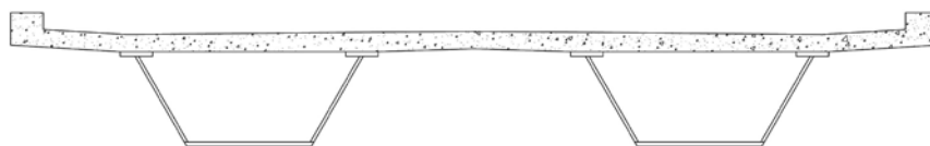
Figure 1 Typical cross section of an open-top composite box girder bridge
