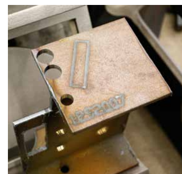
Below: Robotic plasma coping with new plasma etching.
