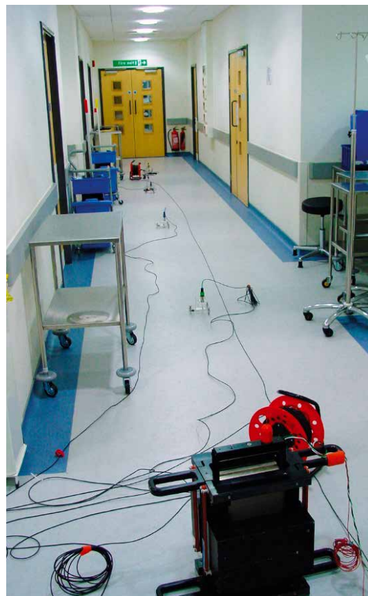
Figure 5: Electromagnetic shaker testing in a hospital corridor.
