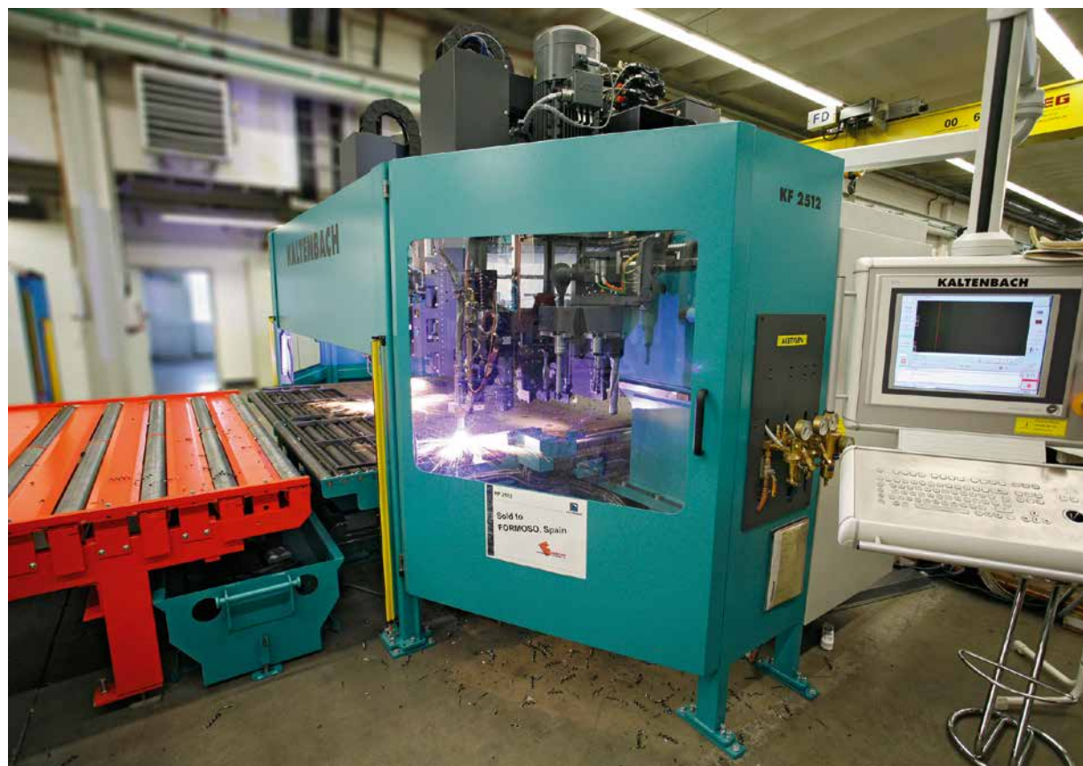
Left: The star of the show - the KVR1001 robotic welder. Below: New high speed plasma plate processing on the KF2512.
