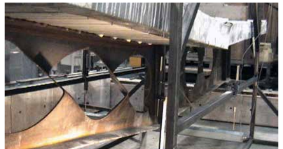
Figure 3: Web post buckling behaviour observed in a cellular beam test. Photograph courtesy Westok Ltd.
