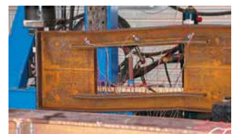
Figure 5: Vierendeel bending of a stiffened rectangular opening.
