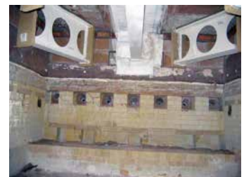
Figure 9: Internal view of the furnace prior to fire testing. Photograph courtesy Leigh's Paints.
