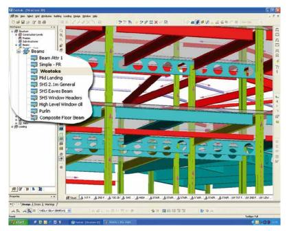
Figure 1: Modelling Cellbeams in CSC FAstrak
