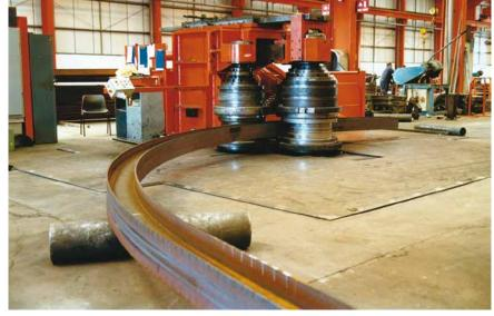
favoured for large sections, especially hollow ones, because the risk of the section distorting or collapsing is greater. "We try to find the most economic solution," says Mr Springthorpe. "For example, with a 300mm square section it may be more economic to increase the wall thickness from 10mm to 12mm and bend it cold rather than keeping the thinner wall and having to hot bend it. There's a large grey area where we offer advice."
