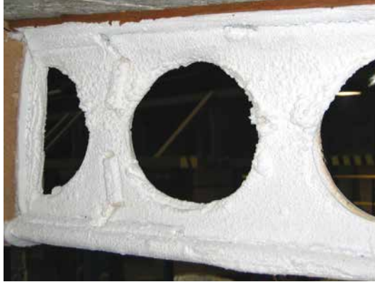
Figures 2 & 3 Unloaded test pieces following the fire test
