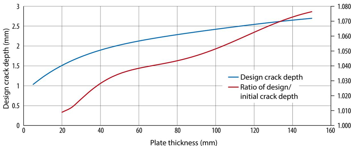
Figure 3: Initial and design crack depths (20,000 cycles)
