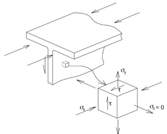
Figure 2: Stresses in plate elements
