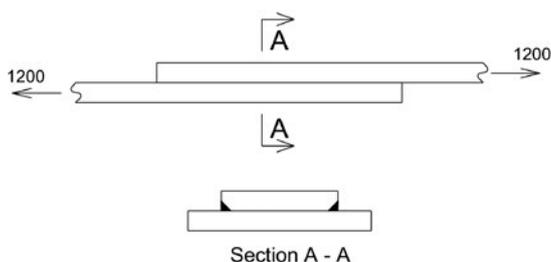
Figure 5: Connection assuming pure shear
