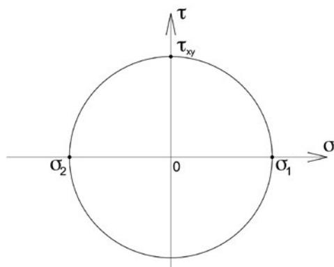
Figure 4: Principal stresses for pure shear
