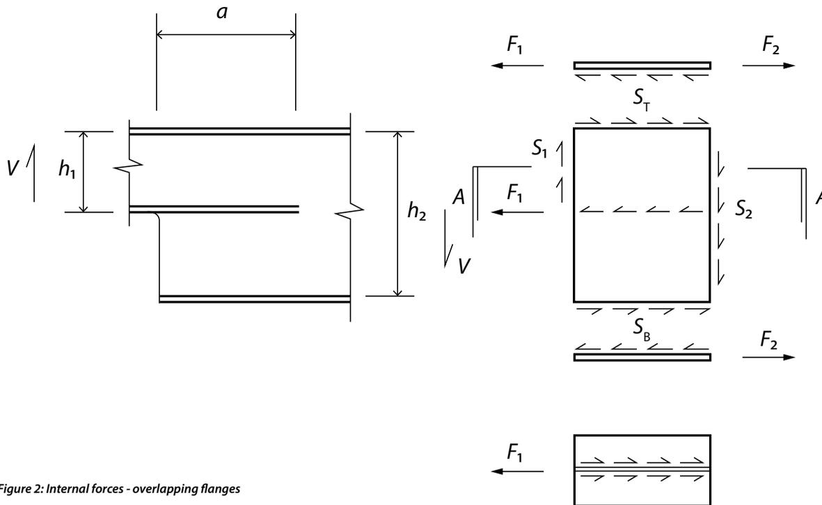
Figure 2: Internal forces - overlapping flanges
