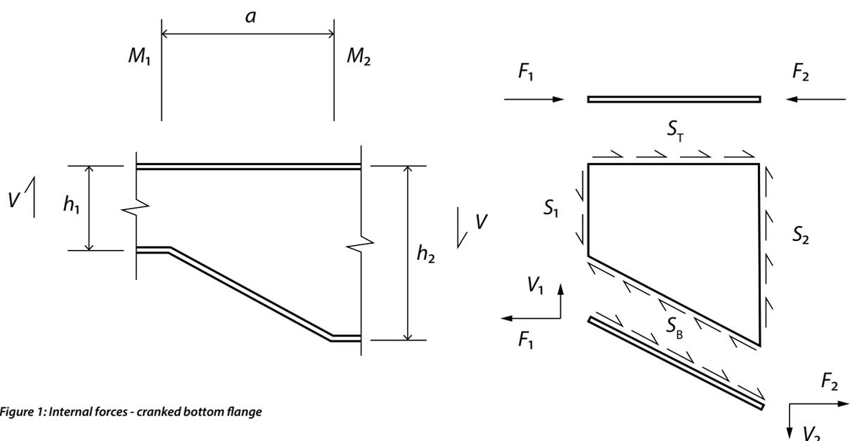
Figure 1: Internal forces - cranked bottom flange
