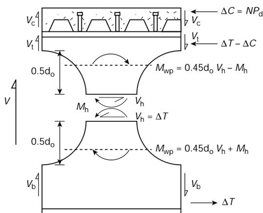
Fig 1. Behaviour of composite asymmetric cellular beams
