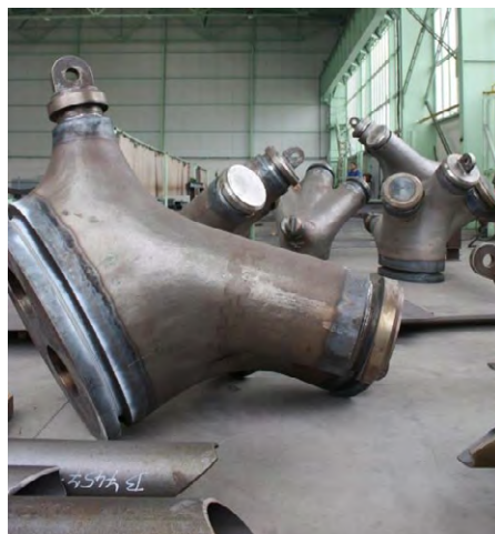
Figure 4: Western Concourse, Kings Cross - steel castings at the fabrication shop © John McAslan + Partners
