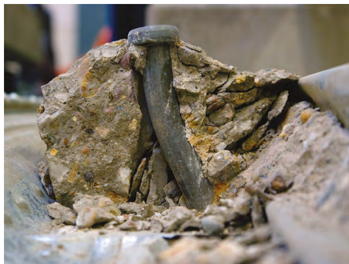
Figure 1: Deformation (slip) of a 19 mm diameter shear stud in transverse decking at failure (courtesy University of Luxembourg)
