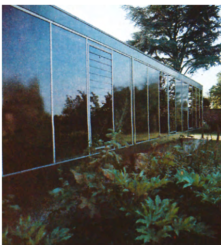
Above and left: A house at Ashted in Surrey constructed on 'legs' with heating-ducts and services suspended in void beneath. Walls are glass panels in patent glazing. Architect: Michael Manser Associates.
