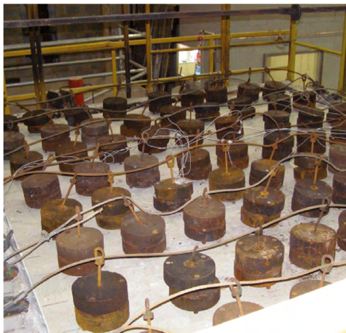
Figure 5: Typical fire test arrangements for a light steel loaded floor
