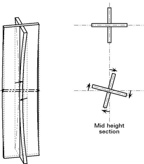
Fig 3. Plain Cruciform deforming in the torsional mode
