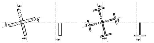
Fig 6. Similarity between torsional buckling and flexural buckling about the minor axis of the component parts
